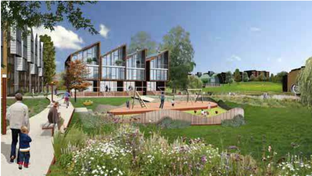
Courtyard rain gardens would slow the passage of rain overland, storing it until the storm has passed
